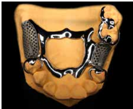
Direct Metal printed dental prosthesis is created rapidly and very accurately in the ProJet 100 dental printing system.
